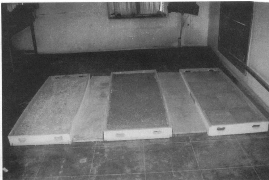
Figure 1. The 3 wooden trays containing pebbles, sand and microcellular rubber, with platforms in between.
