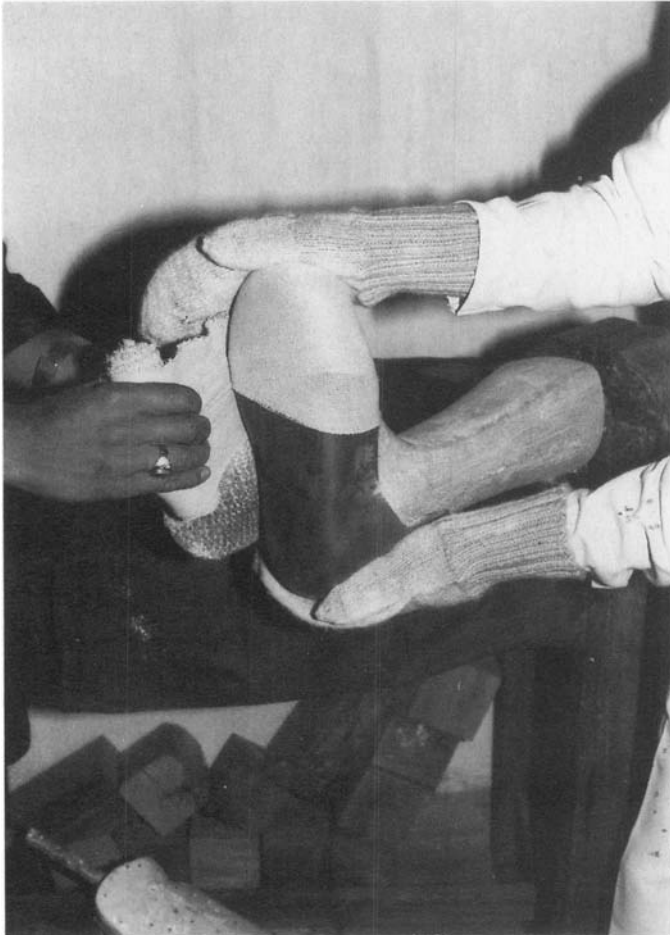
Figure 9. The PVC slab laid over the form and moulded to it with elastic bandage.
